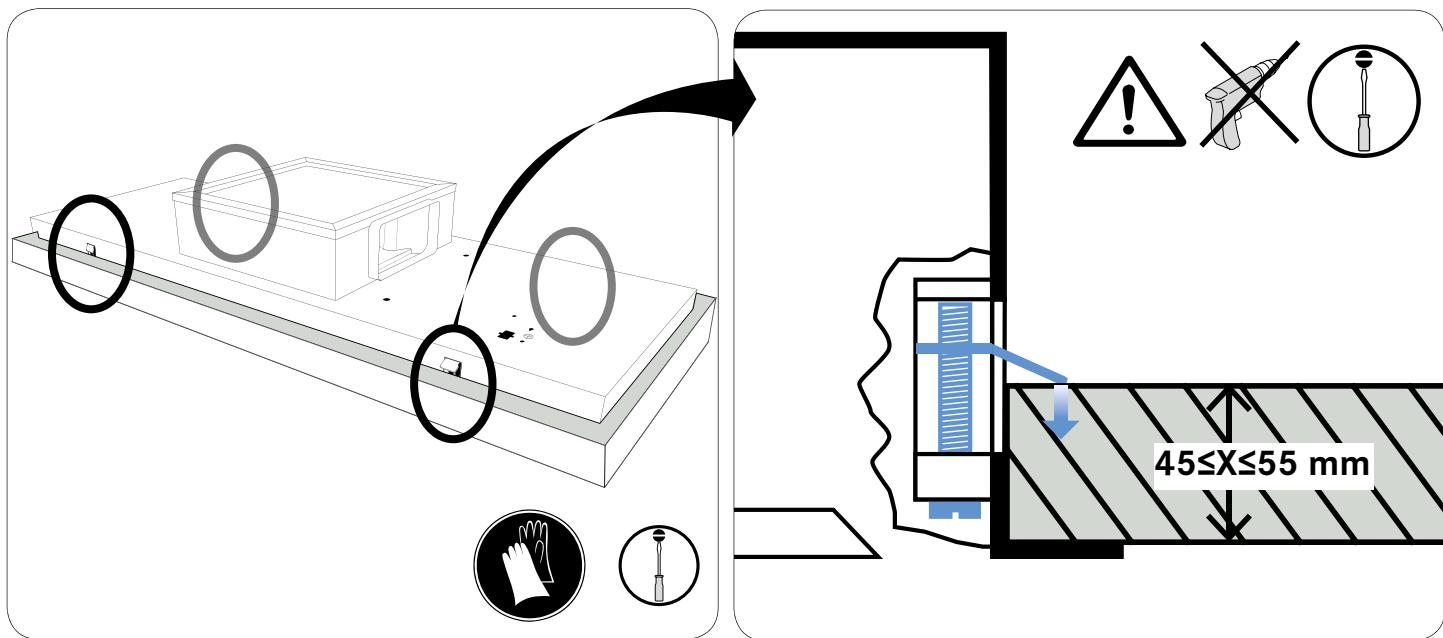
montage - fitting - Montage - montaggio - montaje - Montage
