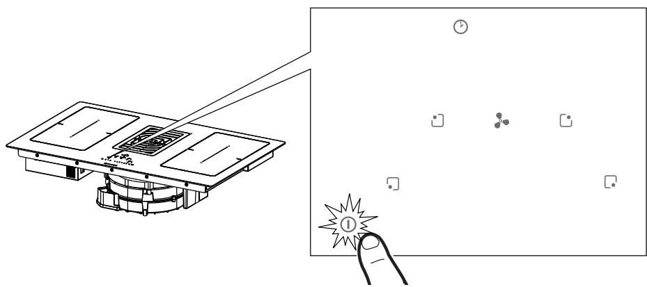
Press and hold the On/Off button ① for 2 seconds to turn the hob on and activate its functions. All the Digits show 8., and the Timer digits show " C L ".
