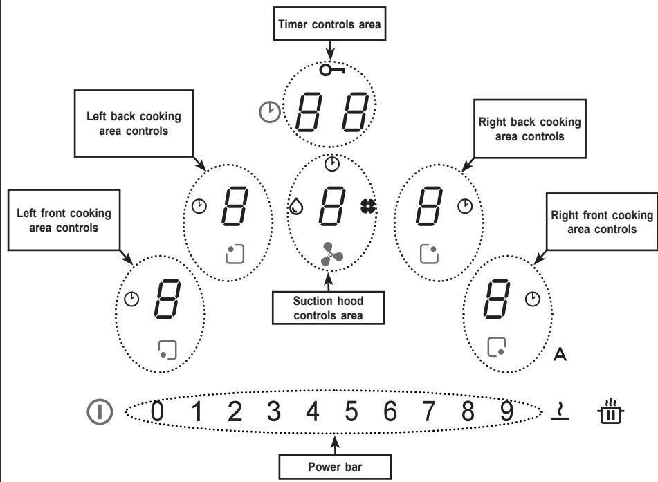
The controls for the cooking areas, suction hood and timer can be activated by pressing on the reference Digit **B**.
