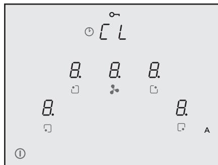
At this point the hob is on but all the cooking areas and the hood are at zero power. The Hob will switch off automatically after 20 seconds if it is not used.
