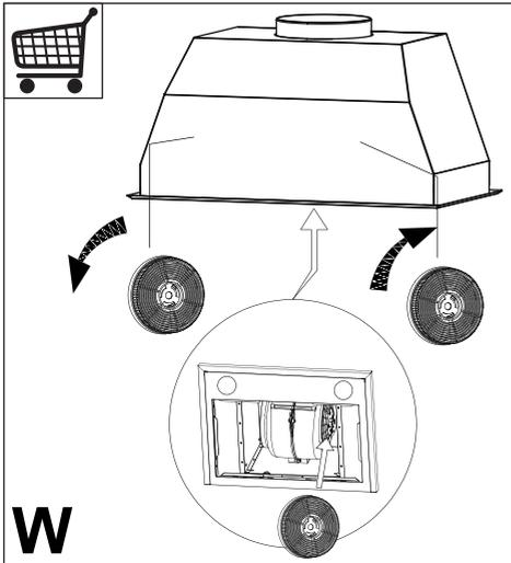
The Grease filters must be cleaned every 1 month of operation, or more frequently for particularly heavy usage, and can be washed in a dishwasher (**Z**).
