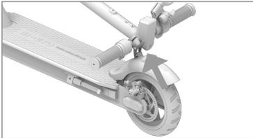
2. Pull up the front tube until it is in vertical position. Close the handle until you hear the click.
