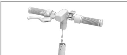
4. Assemble the handlebar with a 3 mm Allen key. Tighten all three screws properly. Screws and tool are included in the box.
