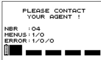
When an error screen is displayed during use, note the error number (in the example, the error number is 1/0/0) and contact the Compex-approved customer service centre.
