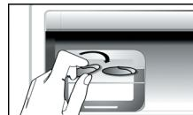
Repeat Step 2 for the other half of the tray, if necessary. To get ice, slightly lift up the storage bin and pull it towards you.
