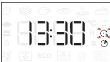
If necessary, turn the knob to set the time you want cooking to end, then press to confirm and start the function.
