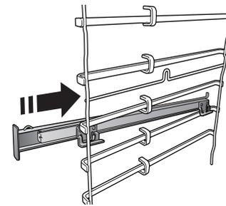
Remove the shelf guides from the oven and remove the protective plastic from the sliding runners.
