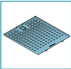
The metal anti-grease filters are there to contain suspended grease particles: deposited on the filters, these feed on any flames released when cooking, generate unpleasant odours, and compromise the passage of air, thus reducing suction performance of the hood.
