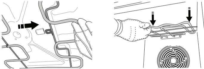
2. To return the heating element to its position, lift it up, pull it slightly towards you and make sure that the tab support is in its proper seating.
