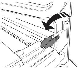
2. Close the door as much as you can. Take a firm hold of the door with both hands – do not hold it by the handle. Simply remove the door by continuing to close it while pulling it upwards (a) at the same time until it is released from its seating (b). Put the door to one side, resting it on a soft surface.
