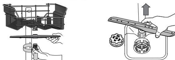
To remove the upper spray arm, turn the plastic locking ring in a clockwise direction.
