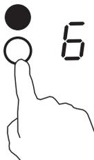
2. Turn the cooking zone off by scrolling down to "0" or touching "--" and "+" control together.
