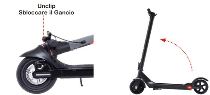
Unclip the hook from the rear Foot Brake.
