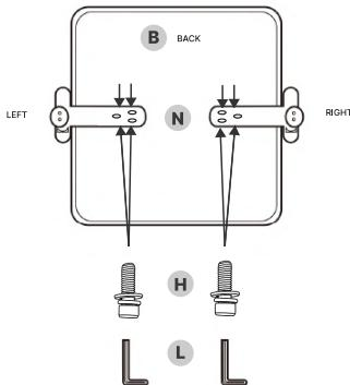
Identify the left and right armsrests (N) and install each on its corresponding side of the seat base (B) using 6 M8X20mm screws (H).
