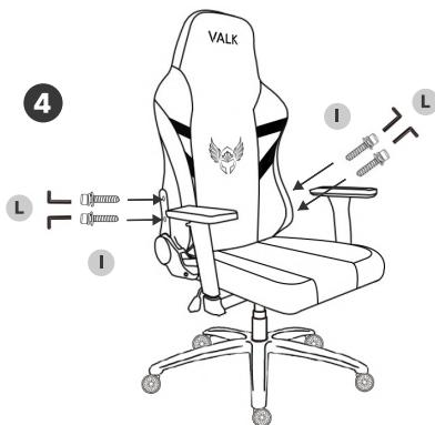
Insert the gas lift (D) into the mechanism housing (C). Fix the backrest (A) to the seat (B) with 4 screws M8×25mm (I).
