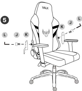
Identify the left and right side covers (K) and install each on its corresponding side of the backrest (A) using 2 M5×8mm screws (J).
