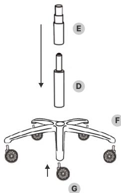
Attach the casters (G) to the base (F). Then put the gas lift (D) in the base (F) and place the cover (E).
