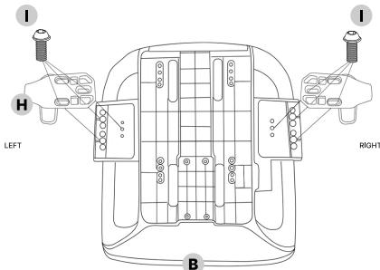
Identify the left and right arms (H) and install each on its corresponding side of the seat base (B) with 6 M6X30mm screws (I).
