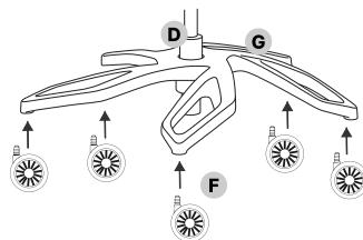
Press the casters (F) into the base (G). Then place the piston (D) in the housing of the base (G).
