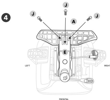
Place the lower part of the backrest (A) on the back of the previously installed mechanism (E) and fix it with 3 M8×25mm screws (J).
