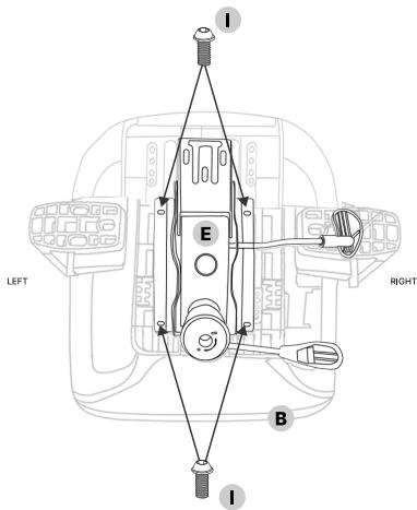
Place the mechanism (E) on the seat base (B) with the adjustment knob facing the front. Match the holes in the mechanism with the pre-installed screws on the seat, and fix it with 4 M6×30mm screws (I).
