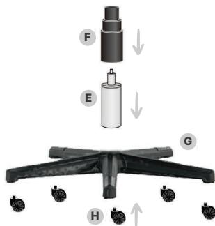
Attach the casters (H) to the base (G). Then put the gas lift (E) in the base (G) and place the cover (F).
