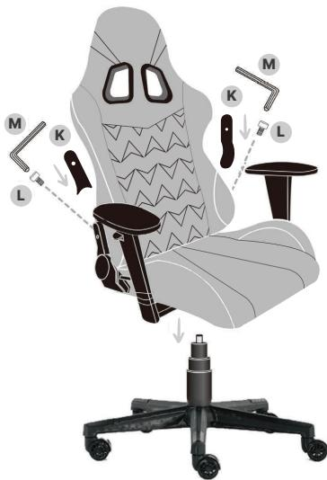
Insert the gas lift (E) into the notch of the mechanism (D) and attach the side covers (K) with 2 M5X8MM screws (L).
