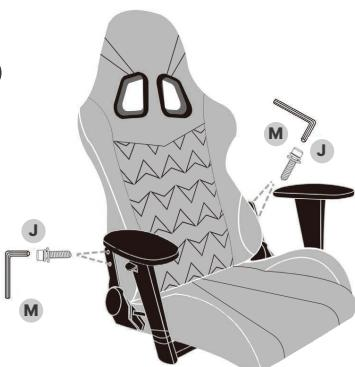
Attach the backrest (A) to the seat (B) using 4 M8x25mm screws (J).
