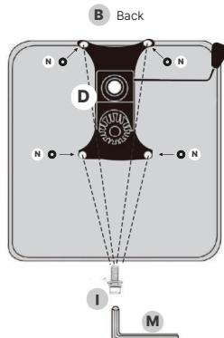
Place the 4 nylon washers (N) over the holes in the base of the seat (B). Install the mechanism (D) on the seat base (B) with 4 M8x20mm screws (I), with the lever facing the back of the seat. Once the chair is assembled, you will operate it with your right hand.
