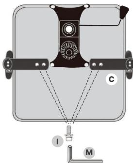
Identify the left and right armrests (C) and install each on its corresponding side of the seat base (B) using four M8x20mm screws (I).
