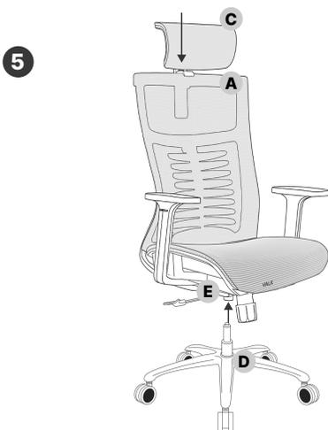
Insert the piston (D) into the mechanism housing (E). Install the headrest (C) by pressing it into the corresponding slot at the top of the backrest (A).
