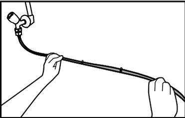
2. Connect the other end of the water hose to the water pump by pushing the hose into the pump's hose inlet.
