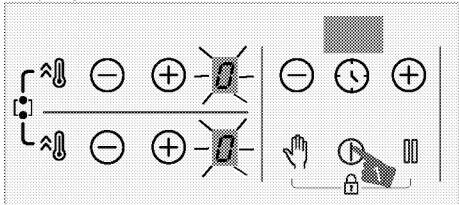
**i** The hob will automatically return to Standby mode if no operation is performed within 10 seconds..
