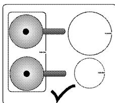
You can use the wide surface cooking zone in two halves separately as rear left and front left cooking zones. Location of the wide surface cooking zone may vary depending on the product model.
