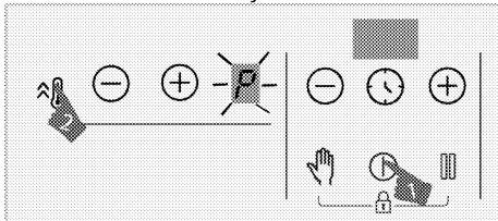
» Selected cooking zone will operate with maximum power and "P" symbol will appear on the cooking zone display. Cooking zone goes out of booster and continues to operate at level "9".
