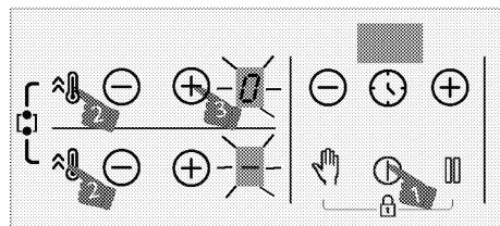
» "0" will appear on the display of the rear-left cooking zone. "⊖" will appear on the display of the front-left cooking zone and the wide surface cooking zone will be activated.
