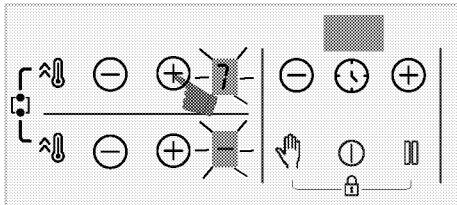
» To change the temperature, touch "⊖"/"⊕" keys of the rear-left cooking zone and set the desired temperature.
