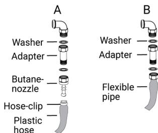
**The butane end piece allows connection using flexible rubber hosing with 6 mm internal diameter suitable for bottle gas.**
