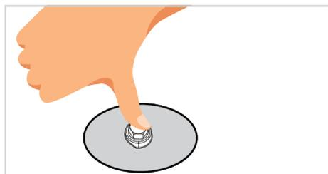
3. Apply prepared soapy water at the injector connection with a small brush, if there is leakage of gas at the injector connection the soapy water will begin to froth. In this case, tighten the injector with a reasonable force and repeat step 3 process once again.
