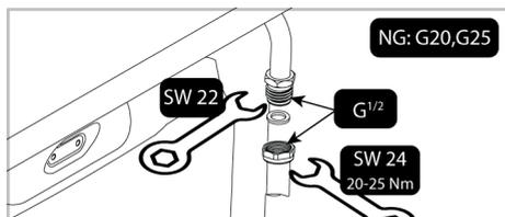
3. You must check for leakage of the connection part after connection.
