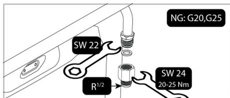
3. Insert the new sealing gasket into the safety gas hose/pipe. Make sure the gasket is seated correctly.
