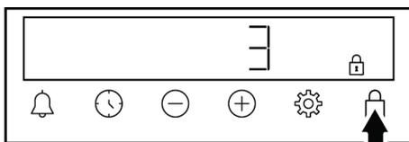
⇒ The 🔒 symbol is shown on the display and the 3-2-1 count down starts. The key lock activates when the countdown ends. When any key is touched after the key lock is set, the timer sounds an audible signal and the 🔒 symbol flashes.
