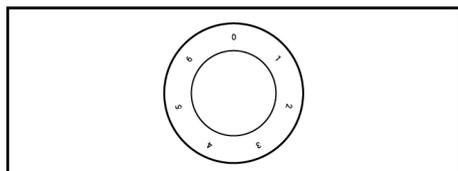
To operate the vitro-ceramic hobs, the hob control knobs are used. To obtain your desired cooking level, switch the hob control knob to the desired level.
