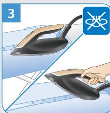
**EN** **Figure 2:** Steam comes out when you move, steam stops when you stop moving or lift up the iron.
