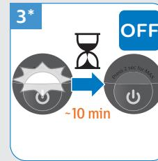
**EN** Figure 3: It switches off automatically when not in use for 10mins.
