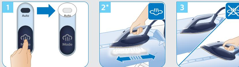
**EN** **Figure 2:** Steam comes out when you move, steam stops when you stop moving or lift up the iron.
