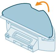
**2** Slide the straight side of the washable mop pad out of the slot.
