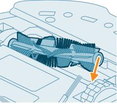
**8** Install the main brush in the correct location. Match the square shaped peg with the square shape hole and insert the brush into position.
