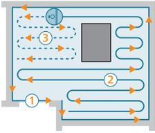
The robot cleans the home in a structured way. The robot cleans room by room and always starts by cleaning the edges of the room first before covering the remaining surface.
