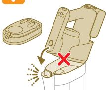
**i** Note: Replace the filter every 6 months to ensure maximum performance. Replacement filters are available under part number XV1791 (see 'Replacement').
