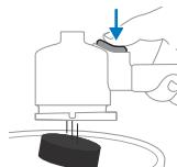
With this ejection button it is very easy to remove the coffee puck after each coffee brew. Remove the coffee puck by holding the portafilter upside down and pressing the ejection button.
