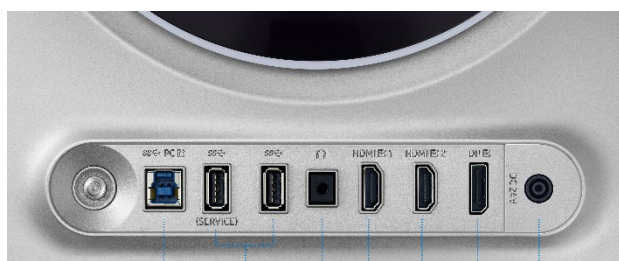
1 PC IN 2 USB/SERVICE 3 Headphone IN 4 HDMI IN 1 5 HDMI IN 2 6 DP IN 7 POWER
