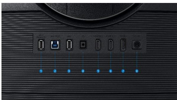
1. USB Type-A Downstream/ SERVICE 2. USB Type-B Upstream 3. USB Type-A Downstream
